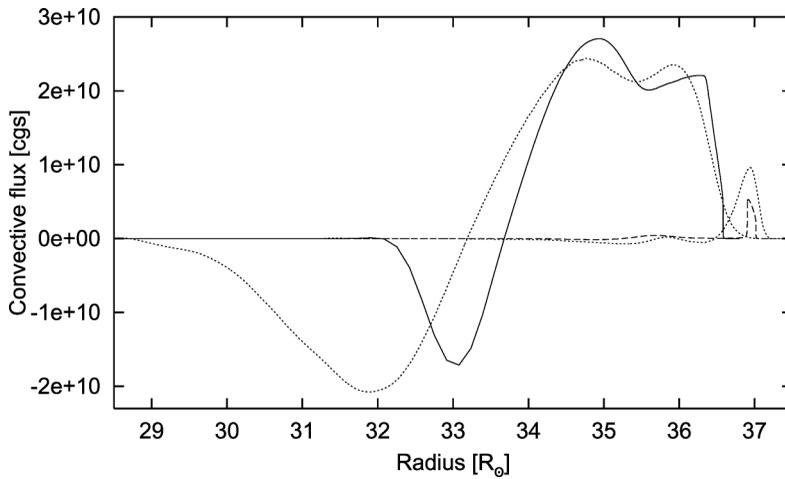
**Figure 3.** Comparison of the two-columns scheme with 2D hydrodynamics. Shown are convective fluxes computed with the two-columns code for Cepheids with effective temperatures of 5200 K (solid line) and 5800 K (dashed line) as well as the corresponding results obtained with CO<sup>5</sup>BOLD (both dotted lines).
