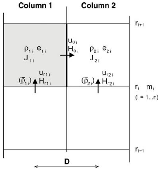
**Figure 1.** The two-columns discretization scheme. The primary variables (compare Table 1) are included in their staggered-mesh localization;  $D$  is the typical distance/diameter of the columns. Advection occurs, as indicated by arrows, in radial direction as well as over the interface between the two columns (thick line).
