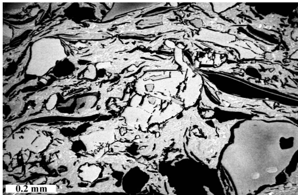
Figure 3 Higher magnification image of the pottery sherd microstructure showing the clay microstructure, which consists of two phases, which is interpreted to result from incomplete transformation to mullite.
