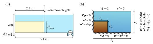
Figure 5. (a) Experimental set-up to study the breaching process. Image taken from Weij (2020). (b) Numerical set-up. In SedFoam, the 'InletOutlet' condition is written as 'pressureInletOutletVelocity' so the velocity is set to have a zero gradient condition when the flow leaves the domain, whereas the velocity assigned when the flow goes into the domain is based on the flux in the patch-normal direction.
