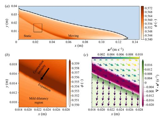
**Figure 3.** (a) Solid volume fraction and zoom-in view along the failure surface with (b) detailed volume fraction and (c) divergence of the solid phase velocity and fluid flow field for the initially loose granular column. It must be noted that the arrows displayed in (c) represent the magnitude of the fluid velocity by their colour and not their size.
