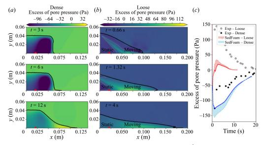
**Figure 4.** Evolution of the morphology and excess of pore pressure  $(p^f)$  during the collapse of an initially (a) dense and (b) loose column. A grey line is included to illustrate the zero pressure isoline. (c) Evolution of basal pore pressure  $(p^f)$  measured at 2 cm (dark continuous line) and 3 cm (light dashed line). Shaded areas correspond to the region between the two probe results.
