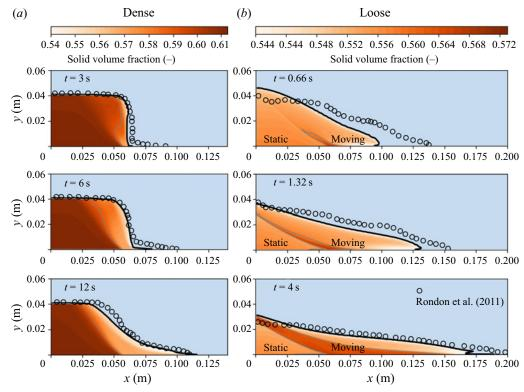
**Figure 2.** Evolution of the morphology and solid volume fraction during the collapse of an initially (a) dense and (b) loose column. A grey line is included to illustrate the evolution of the isoline with the initial volume fraction ( $\phi_o = 0.55$  for the initially loose column and  $\phi_o = 0.61$  for the initially dense column).
