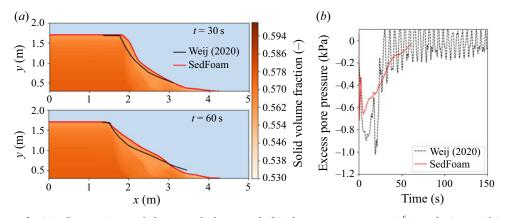
**Figure 8.** (a) Comparison of the morphology and (b) the pore pressure  $(p^f)$  evolution within the granular column between the experiments and the numerical simulations for the D9 sand.
