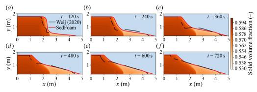
Figure 6. Comparison of the morphology between the experiments and the numerical simulations for the GEBA sand.
