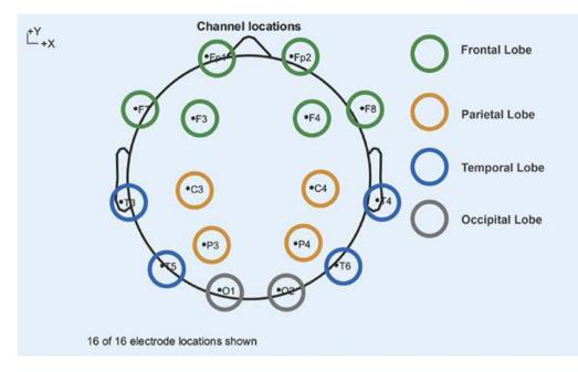
Fig. 6. Neurofax EEG-9200 system with 16 scalp and 2 mastoid Ag/AgCl electrodes mounted according to the 10/20 system, and the relations between 16 channels and brain area.
