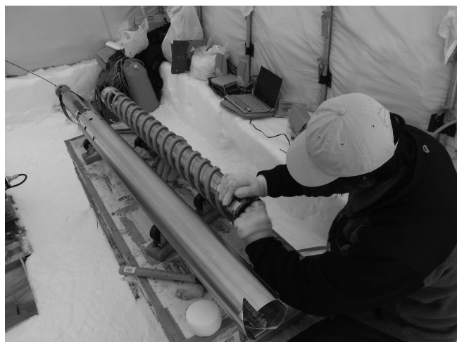
Fig. 2. Drill jacket and barrel of Geotech Co. Ltd used at Ichinsky and Aurora Peak.
