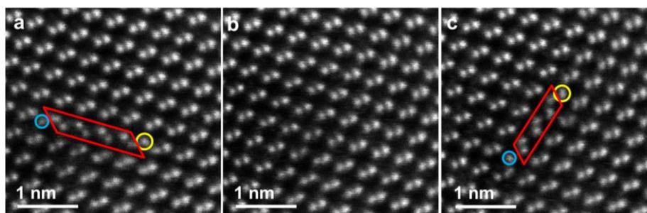
**Figure 3.** (a) STEM Z-contrast image shows unpaired Cd (blue circle) and Te (yellow circle) columns in a dislocation pair associated with an intrinsic stacking fault (red frame). The dislocation pair can (b) annihilate and (c) reappear with a stacking fault in another direction (submitted for publication).
