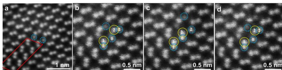
**Figure 2.** (a) STEM Z-contrast image shows two unpaired Cd (blue dashed circles) in a 90° Shockley partial dislocation associated with an extrinsic stacking fault (red frame). (b-d) 3 continuous frames from a movie showing the partial dislocation gliding back and forth along the stacking fault. The blue and yellow circles indicate Cd and Te columns, respectively (submitted for publication).
