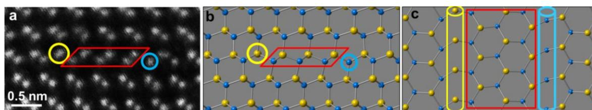
**Figure 1.** (a) STEM Z-contrast image showing unpaired Cd (blue circle) and Te (yellow circle) columns in the dislocation pair associated with an intrinsic stacking fault. (b) Corresponding model built with DFT. (c) The side view of the dislocation plane shows that no dimer is formed along the dislocation. The red frames indicate the intrinsic stacking fault.
