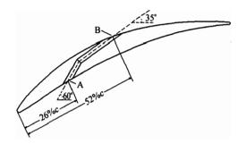
Figure 1. Convergent turning slot of two-segments [12].
