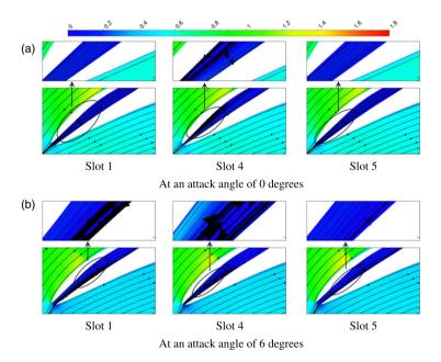
Figure 11. Mach number contours near the leading edges.
