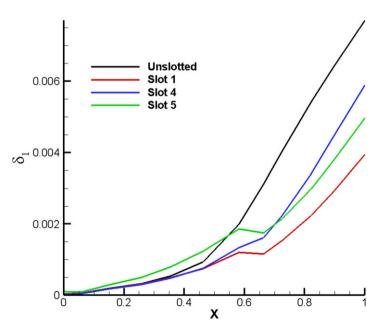
*Figure 13.* Distribution of the thickness of the boundary layer on the suction surface at an attack angle of 6 degrees.
