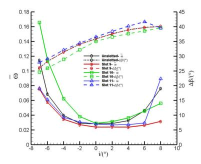
Figure 22. Performance of cascades with different slot outlet locations.
