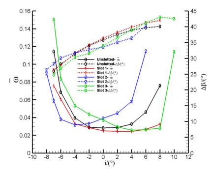
Figure 8. Performance of cascades with different slot inlet locations.
