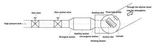
Figure 26. Structure of the experiment bench.
