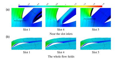
Figure 12. Mach number contours at an attack angle of 6 degrees.
