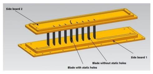
Figure 28. Three-dimensional view of the cascade.
