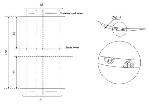
Figure 27. Schematic diagram of static pressure holes drilled on the blade.
