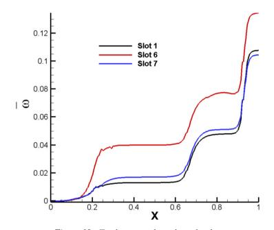
Figure 18. Total pressure loss along the slot.
