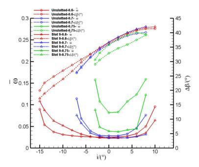
Figure 23. Performance of slotted and unslotted cascades at various inlet Mach numbers.
