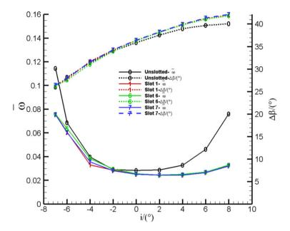
Figure 16. Performance of cascades with different slot shapes.
