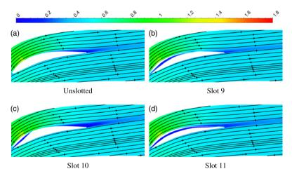
Figure 20. Mach number contours at an attack angle of 0 degrees.
