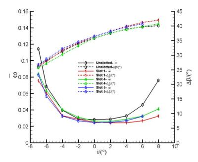
Figure 14. Performance of slotted cascades with different slot inlet widths.
