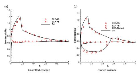
Figure 31. Distribution of the isentropic Mach number on the blade surfaces.
