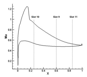
*Figure 21.* Distribution isentropic Mach numbers on the surfaces of an unslotted blade and the outlet slot positions.
