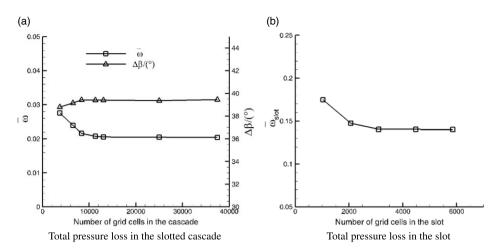
Figure 30. Total pressure loss varies with the number of grid cells.
