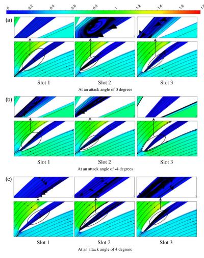
Figure 9. Mach number contours near the leading edges.
