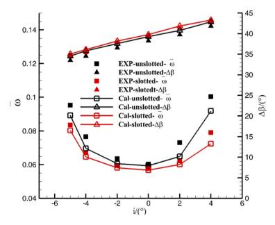
Figure 32. Performance of the unslotted and slotted cascades.
