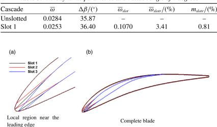
Table 3. Aerodynamic parametres at an attack angle of 0 degrees
