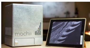
**Figure 1.** (left) Voxa's *Mochii*<sup>TM</sup> Electron Microscope (left) with iPad controller (right) showing a high resolution image of the head of a wheat plant [1].
