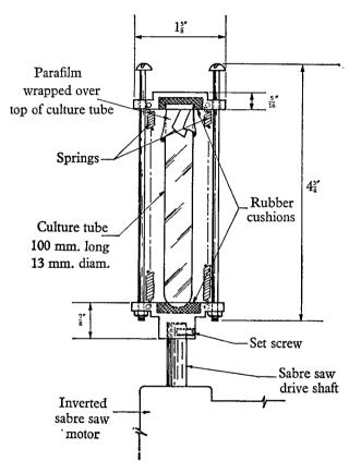
Fig. 1. Diagram of blendor showing essential parts and typical dimensions.
