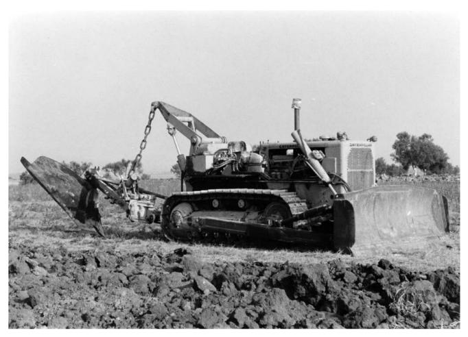
FIGURE 1.15 Deep-ploughing technology used in the countryside around Tuscania at the time of the fieldwork. (Photograph: Graeme Barker.)
