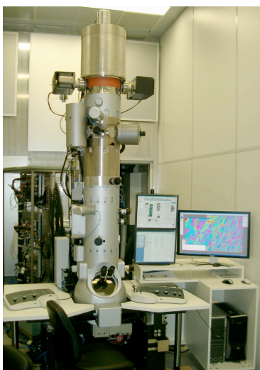
Figure 2. Monochromated, aberration-corrected TEM with in-column energy filter, as developed from the Zeiss Libra 200 MC platform
