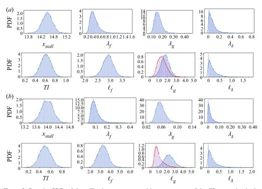
Figure 5. Posterior PDFs of the calibration parameters and hyperparameters of the GPs appearing in the HC-MFM (2.6) for (a)  $C_L$  and (b)  $C_D$ . Associated training data and predictions are shown in figure 4. In the plots of  $\ell_g$ , the blue and red histograms correspond to the AoA and TI, respectively. Note that the values of TI are in percentage.
