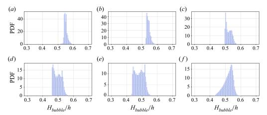
Figure 10. (a-e) The PDF of  $H_{bubble}/h$  at x/h=2.5 due to the variation of  $\alpha$  and  $\gamma$  using the RANS data simulated with  $\kappa$  equal to 0.348, 0.367, 0.400, 0.433, 0.452, respectively. Note that  $5 \times 5$  samples are taken from the  $\alpha-\gamma$  space at each of these constant- $\kappa$  simulations. The PDF in (f) is obtained using all the  $5 \times 5 \times 5$  samples from  $\alpha$ ,  $\gamma$  and  $\kappa$ .
