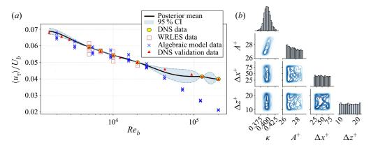
Figure 3. (a) Mean prediction of  $\langle u_{\tau} \rangle / U_b$  and associated 95 % CI along with the training data and validation data from DNS of Iwamoto *et al.* (2002), Lee & Moser (2015) and Yamamoto & Tsuji (2018), (b) diagonal, posterior density of parameters  $\kappa$ ,  $A^+$ ,  $\Delta x^+$  and  $\Delta z^+$ ; off diagonal, contour lines of the joint posterior densities of these parameters. The value of the contour lines increases from the lightest to darkest colour.
