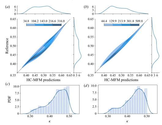
Figure 13. (a,b) Joint and marginal PDFs of  $H_{bubble}/h$  at x/h = 2.5, and (c,d) associated sample posterior distribution of  $\kappa$  for (a,c) case-A and (b,d) case-B data sets. In (a,b), the contours belong to the joint PDF with associated values specified in the colour bar.
