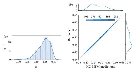
Figure 8. (a) The sample posterior PDF of  $\kappa$  and (b) sample joint PDF of  $H_{bubble}/h$  at x/h=2.5 obtained from the HC-MFM using all nine DNS data sets of Xiao *et al.* (2020) along with the 125 RANS simulations performed in the present study. The RANS simulations are performed using five samples of  $\kappa$  equal to 0.348, 0.367, 0.4, 0.433 and 0.452. The marginal PDFs on the top and right axes are found using the kernel density estimation method.
