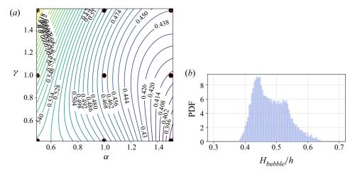
Figure 7. (a) Isolines of the response surface and (b) PDF of  $H_{bubble}/h$  at x/h = 2.5 due to the variation of  $\alpha$  and  $\gamma$  using all of the nine DNS data of Xiao et al. (2020) (represented by the symbols in the left plot). These plots are considered as ground truth or reference for evaluating the performance of the MFM.
