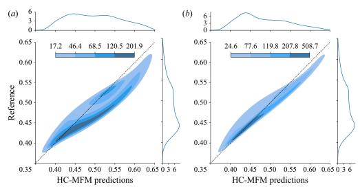
Figure 15. Joint and marginal PDFs of  $H_{bubble}/h$  at x/h = 2.5 for (a) case-A and (b) case-B data sets. Here, a MAP estimator is used to construct the HC-MFM, in contrast to figure 13 and the rest of the examples in the present study which are obtained using an MCMC method.
