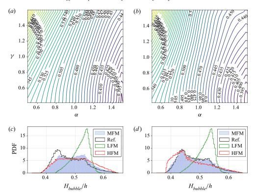
Figure 12. (a,b) Isolines of the response surface and (c,d) PDF of  $H_{bubble}/h$  at x/h = 2.5 due to the variation of  $\alpha$  and  $\gamma$  obtained from the HC-MFM with the data of (a,c) case-A and (b,d) case-B. In (c,d), the PDF resulting from the HC-MFM is compared with the PDFs of the ground truth (see figure 7), LF data (LFM, figure 10) and HF data (HFM, figure 11).
