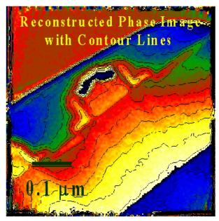
FIG. 3b. Reconstructed phase image of transistor region, useful for dopant profiling.
