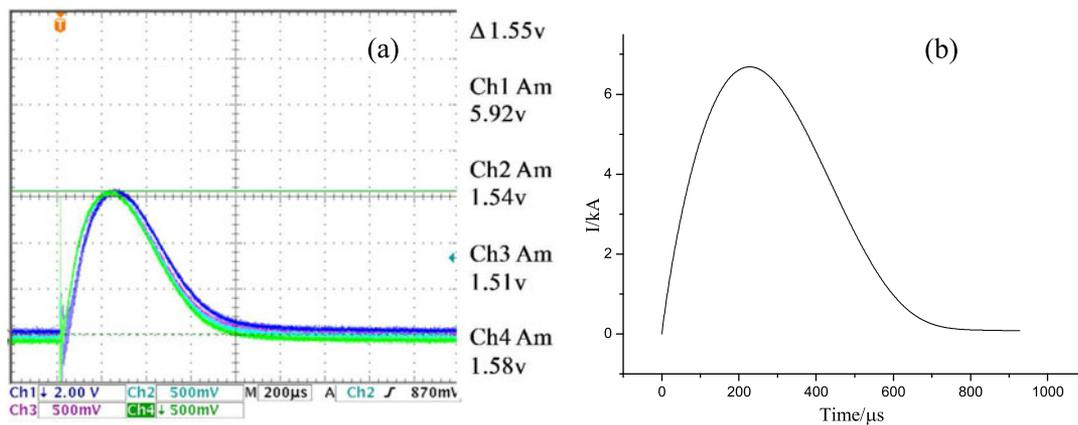
Figure 5. Current pulse shape: (a) experimental result; (b) calculated result.
