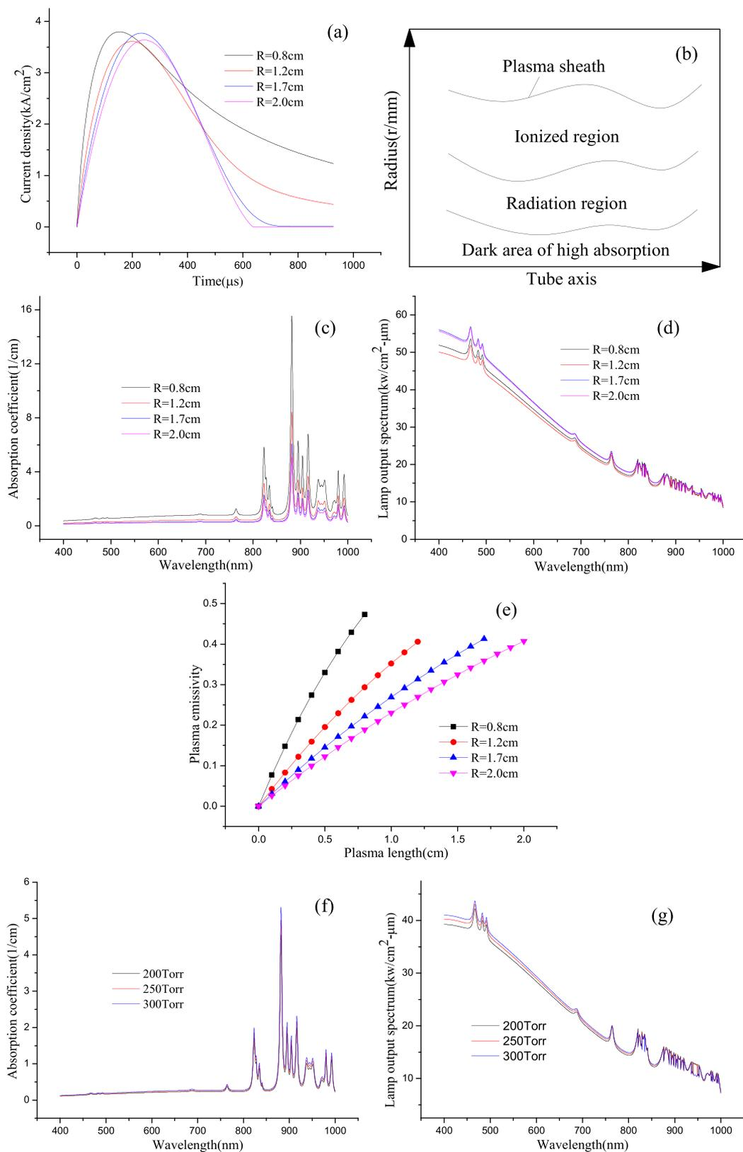
**Figure 3.** Effect of lamp diameter and xenon pressure on the absorption coefficient: (a) current pulse shapes at different xenon lamp diameters; (b) schematic diagram of xenon plasma; (c) absorption coefficient; (d) lamp output spectrum; (e) plasma emissivity for  $\lambda = 700$  nm at different xenon lamp diameters; (f) absorption coefficient at different xenon pressures; (g) lamp output spectrum.
