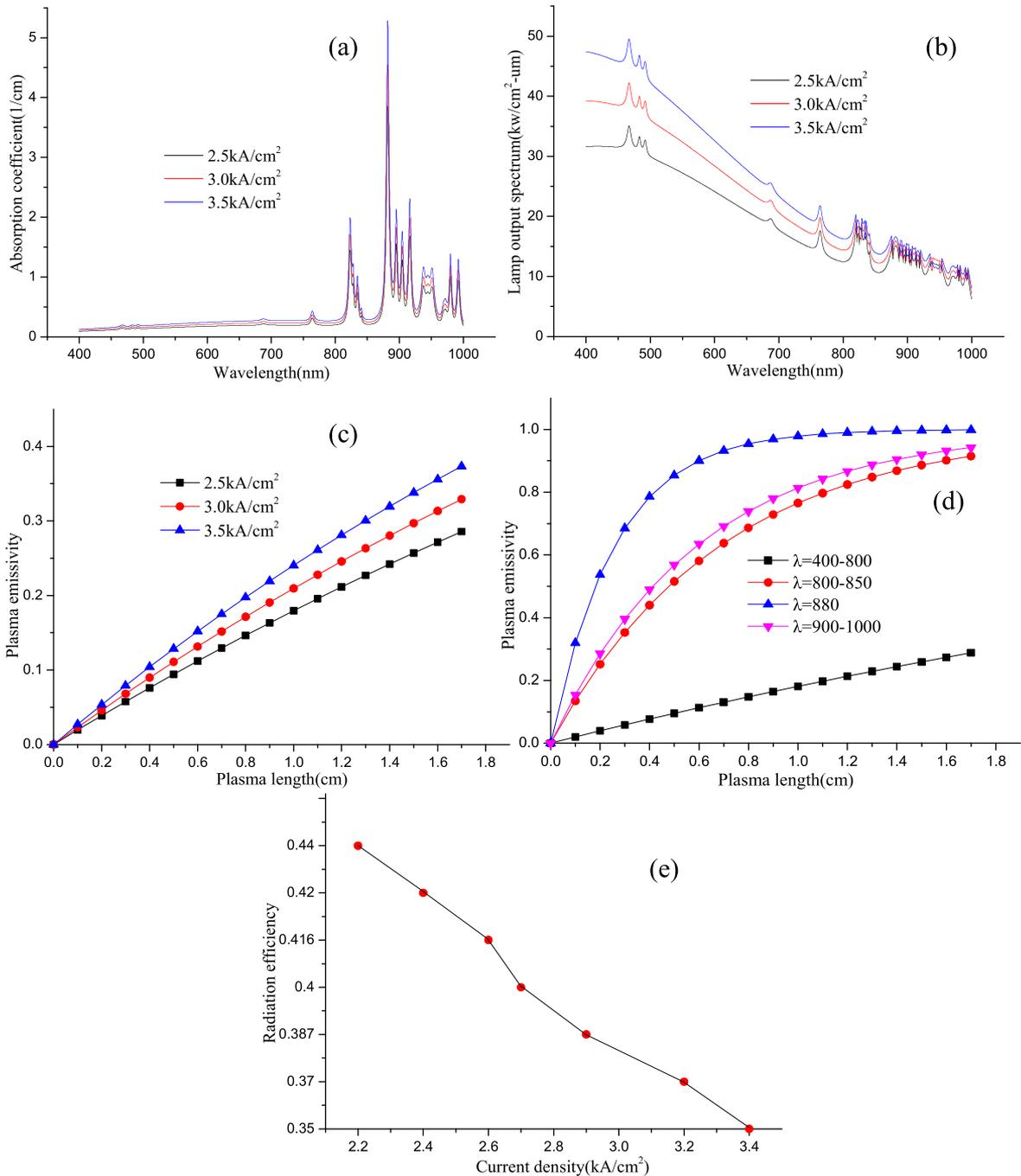
**Figure 2.** Effect of current density on the xenon flash lamp absorption coefficient: (a) absorption coefficient; (b) lamp output spectrum; (c) plasma emissivity at different current densities with the same wavelength; (d) plasma emissivity at different wavelengths with the same current density; (e) relationship between current density and radiation efficiency.
