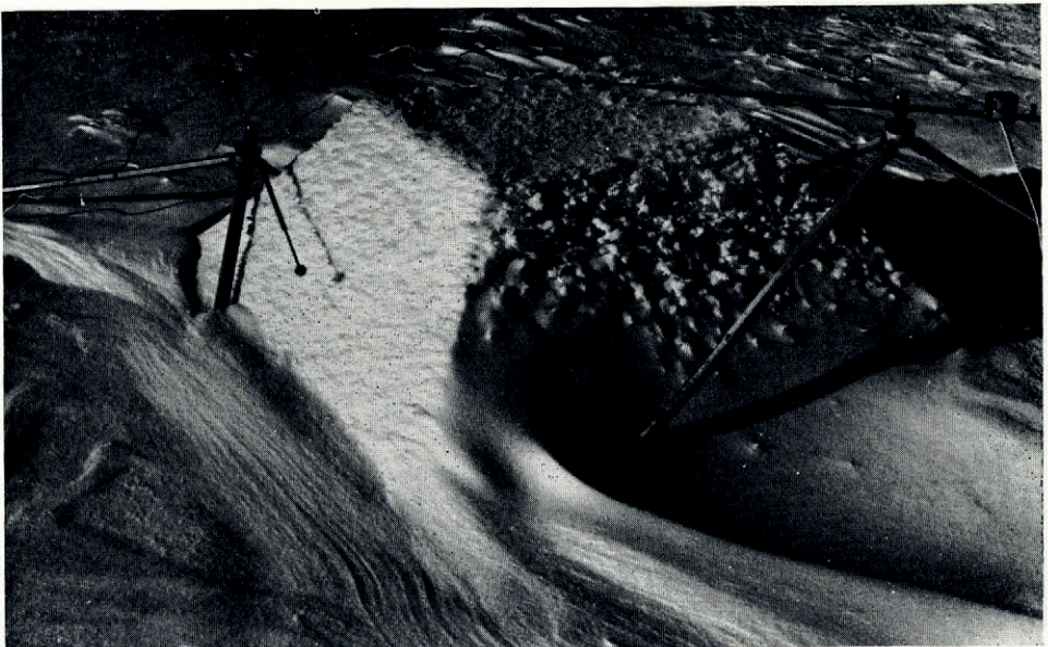
Fig. 6. The snow block after a period of light snowdrift, with the miniature net radiometers in position.
