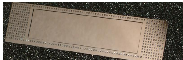
Fig. 3: High purity silicon detector thinned down to a thickness of 50 \mu\text{m} . The detector properties remain unchanged [3].
