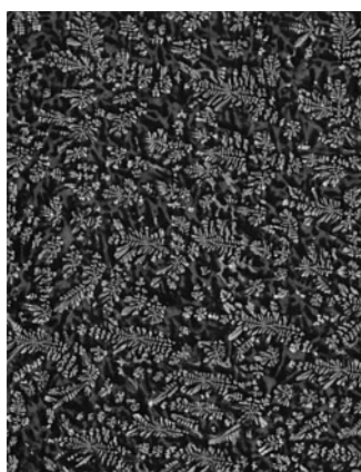
On the Cover: Backscattered electron image of Mg 45 –Al 28 –Zn 27 alloy at 20 kV from Teng, et al, page 58.
