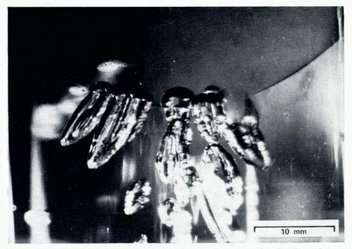
Fig. 18. Large air bubbles formed from water saturated at 850 mbar, frozen at 500 mbar. Growth rate: 6 µm s<sup>-1</sup>.
