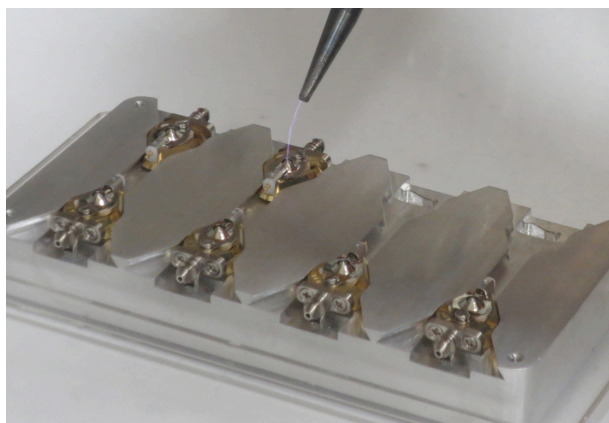
Figure 1. Restoring local electrode performance by applying electric discharges from a hand-held Tesla coil. Photo credit: Stoichko Antonov.
