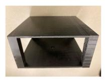
Figure 6. The 3D printed table for holding the ArUco marker.
