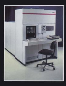
The Model 4175 Rutherford Backscattering Surface Analyzer is a compact, easy to operate instrument, designed for routine surface and depth characterization of thin films and solid materials. Rutherford Backscattering provides:
