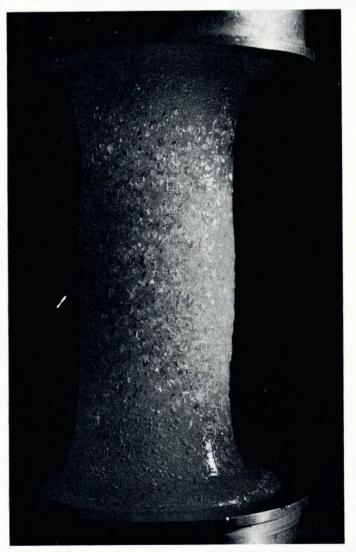
Fig. 15. Dumbbell compression specimen after failure. The center section is filled with internal cracks. At an earlier stage in the deformation, such specimens develop a lumpy surface as surface grains bulge out.
