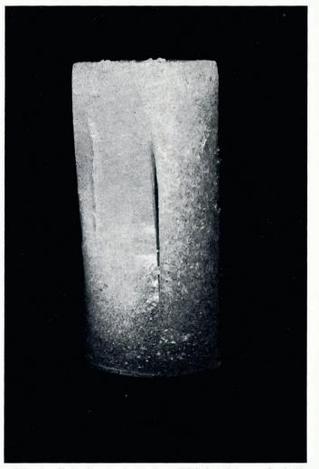
Fig. 17. Axial cleavage failure in cylindrical compression specimen. With the technique employed, this was the usual mode of failure for simple cylindrical specimens.
