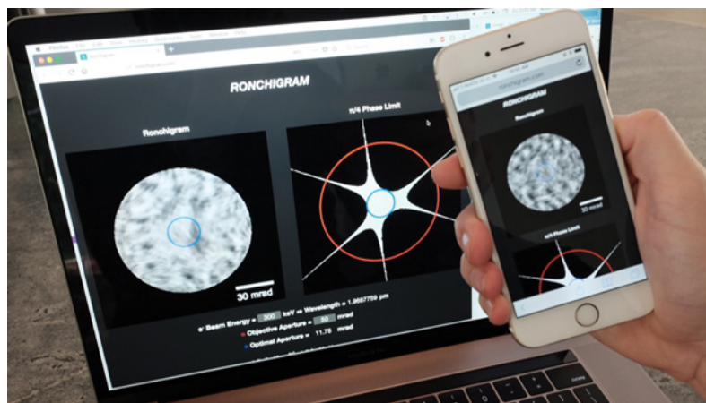
Figure 3: The Ronchigram.com web application allows exploration of Ronchigrams on any laptop computer or mobile phone. The blue circle visible in the Ronchigram on the phone indicates the maximum aperture size for the highest resolution achievable.
