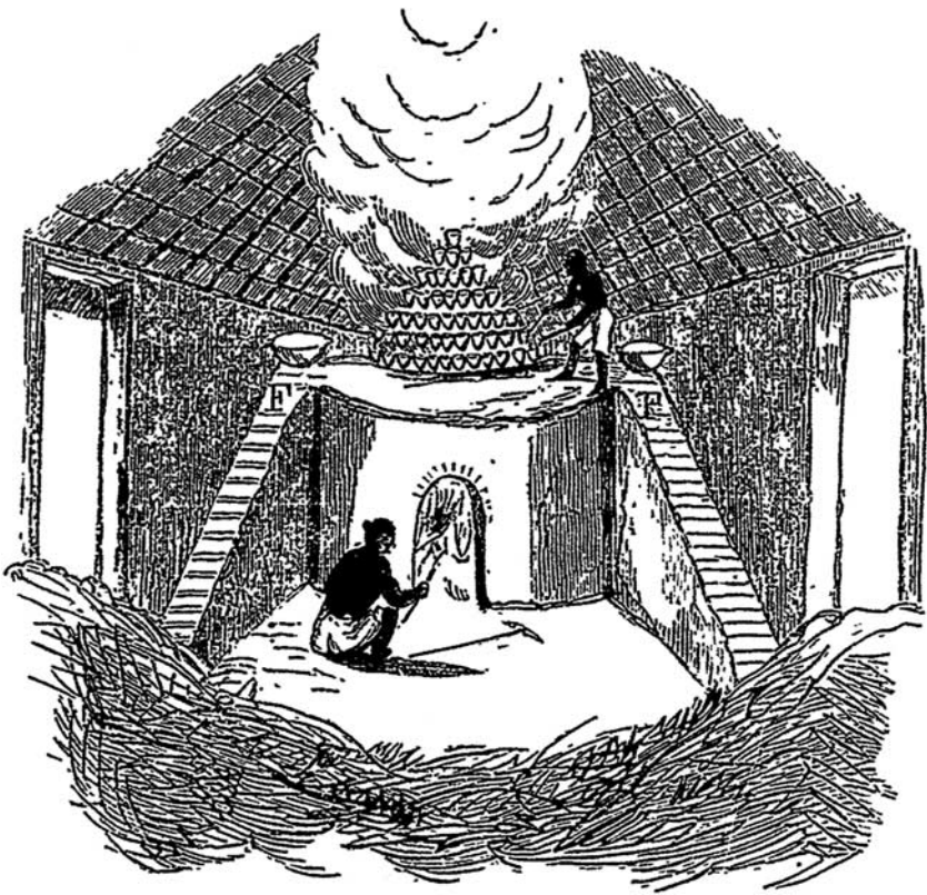
Figure 2. The interior of a boiling house in Tamluk, with two malangis boiling brine with grass or paddy straw.
