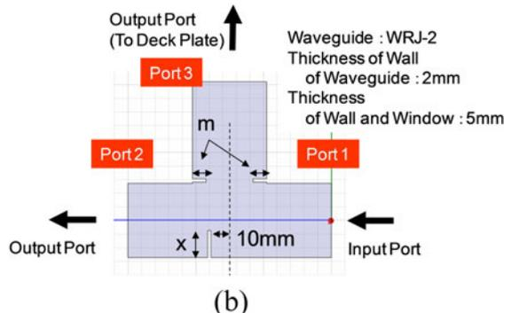
Fig. 5. (a) Photograph and (b) illustration of the developed power divider.
