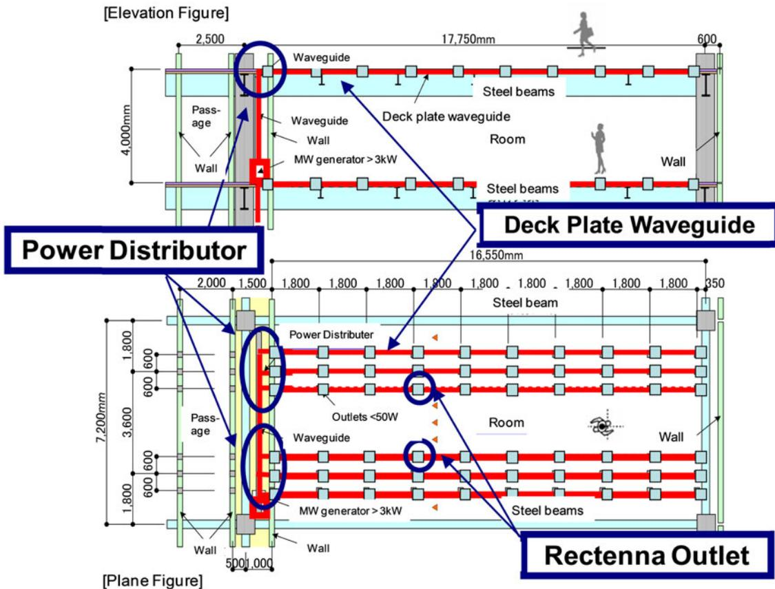
Fig. 2. Elevation and plane diagrams of the WPDS.
