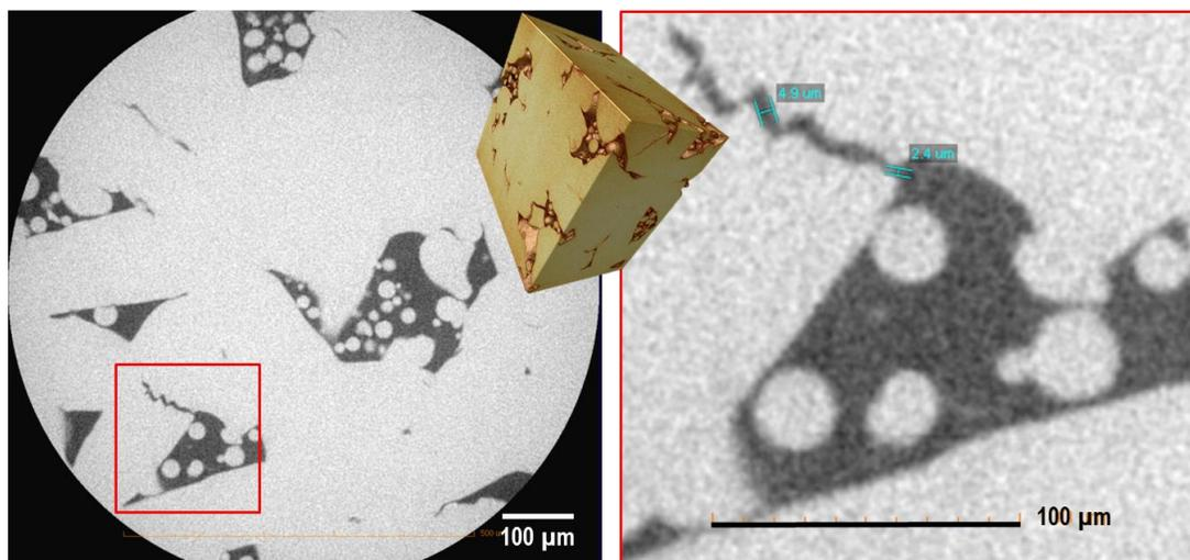
**Figure 1** From the 3D reconstructed dataset (inset), a virtual 2D cross-section (left) reveals several regions of non-sintered powder steel volume. In addition to the non-sintered volume, several micron-size cracks were discovered. Sample courtesy of NIST.
