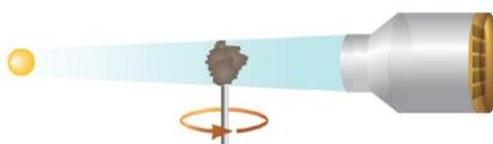
**Figure 2** Sub-micron XRM (ZEISS Xradia Versa) optical architecture. Magnification is achieved through a combination of geometric (sample, source, detector placement) and optical (post-sample, variable scintillator-lens-ccd coupling) methods.
