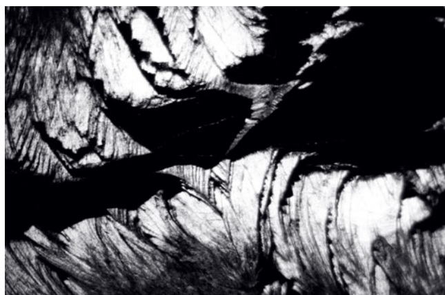
Fig. 11. Close-up of cone-in-cone structure in the periphery of two spherules.
