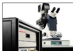
Leica launched the Leica SR GSD 3D, a widefield system that not only offers 2D, but now also 3D super-resolution imaging of molecules and cellular structures. Based on Ground State Depletion, the widefield fluorescence microscope attains resolutions of down to 20 nm in the lateral and 50 nm in the axial direction. The Leica SR GSD 3D also scores with its unique precision for localizing single molecules, its system stability, and its optical performance.
