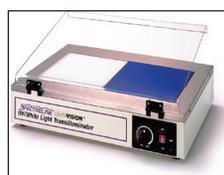
The advanced Spectroline® Bi-O-Vision™ Series transilluminators feature two workstations, producing both 312 nm ultraviolet and white light. The TD-1000R model offers fixed-intensity, whereas the TVD-1000R model offers variable-intensity control of either UV or white light. These units are continuously adjustable from 100% down to 50%. This enables life science researchers to select medium wavelength ultraviolet or white light illumination to view fluorescent gels or visible blots.
