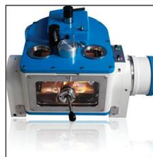
The PP3010T is a highly automated, easy to use, column-mounted, gas-cooled cryo preparation system suitable for most makes and models of SEMs, FE-SEMs, and FIB/SEMs. The PP3010T has all the facilities needed to rapidly freeze, process, and transfer specimens. The cryo preparation chamber is turbomolecular-pumped and includes tools for cold fracturing, controlled sublimation, and specimen coating. The specimen can then be transferred onto a highly stable SEM cold stage for observation.
