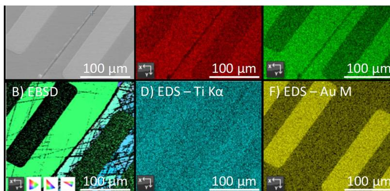
**Figure 2.** A) Secondary Electron image of electrodes patterned across a grain boundary and B) the electron backscattered diffraction (EBSD) map showing the change in grain orientation between metal electrode contacts. C-F) Energy Dispersive Spectroscopy (EDS) of the same area revealing the Au contacts are resting on either side of a  $\text{Bi}_2\text{Te}_3$  grain boundary, with no composition difference between the two grains.
