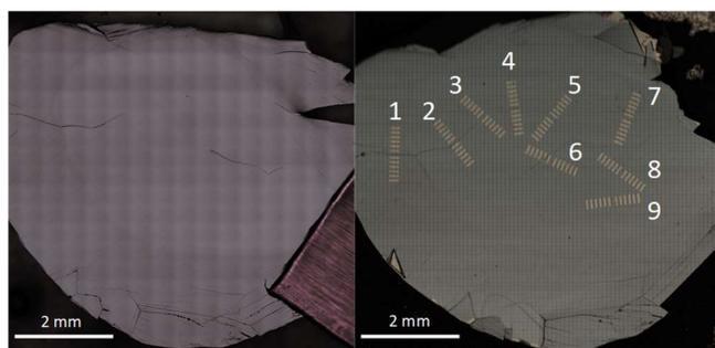
**Figure 1.** Optical montage images of a 50  $\mu\text{m}$  thick  $\text{Bi}_2\text{Te}_3$  thermoelectric (left) before and (right) after Au contacts were deposited across 9 different grain boundaries. These boundaries were located using EBSD.
