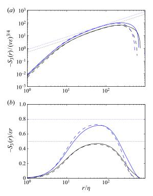
Figure 6. Comparison of third-order structure functions in DNS (solid lines) and EDQNM (short dashed lines) for three (blue) and four (black) dimensions: (a) scaled by appropriate Kolmogorov quantities; (b) scaled by energy dissipation and r. In (a) the dotted lines correspond to the expected 12r/d(d+2) inertial range scaling behaviours whilst in (b) they are for the values 12/d(d+2).
