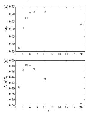
Figure 5. (a) EDQNM velocity derivative skewness vs dimension. (b) Enstrophy production term  $-S_0\Lambda(d)$  vs dimension.
