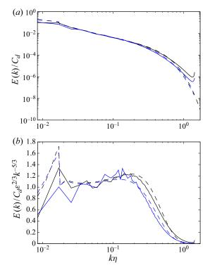
Figure 1. (a) Comparison between DNS (solid lines) and EDQNM (dashed lines) of energy spectra scaled by the Kolmogorov microscale,  $\eta$ , for three (blue) and four (black) dimensions. (b) Compensated energy spectra for the same data.
