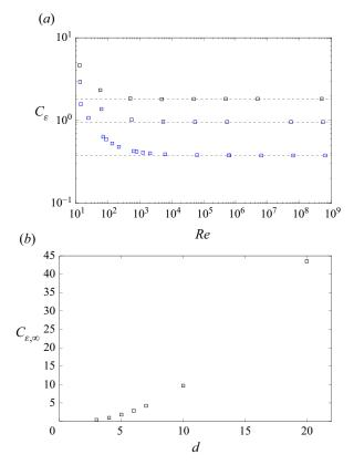
Figure 8. (a) Plot of  $C_{\varepsilon}$  vs Re for three, four and five dimensions, darker colour indicates higher dimension with five dimensions in black. Dashed lines indicate the value for  $C_{\varepsilon,\infty}$ ; (b)  $C_{\varepsilon,\infty}$  against spatial dimension, d.
