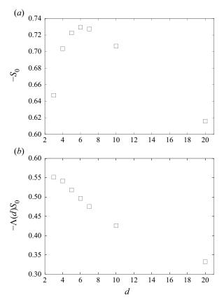
Figure 9. (a) EDQNM velocity derivative skewness vs dimension for  $C_d = 1$  runs. (b) Enstrophy production term  $-S_0 \Lambda(d)$  vs dimension for  $C_d = 1$  runs.
