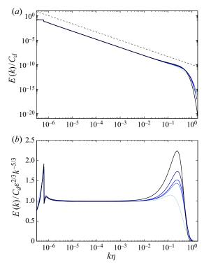
Figure 2. (a) EDQNM energy spectra scaled by the Kolmogorov microscale,  $\eta$ , for three, six, seven, ten and twenty dimensions, the darker the shade of the line the higher the dimension with twenty being black. Dashed line shows  $k^{-5/3}$  scaling. All dimensions have the same viscosity and energy dissipation. (b) Compensated spectra for the same data, colours the same.
