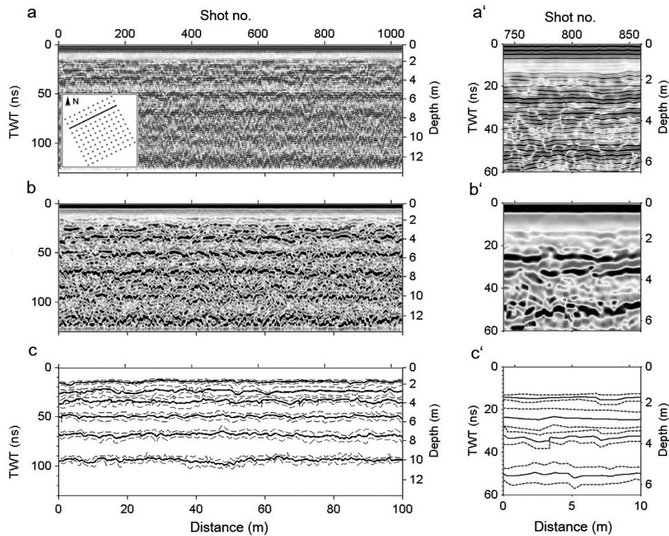
**Fig. 2.** Sample 500 MHz GPR profile, aligned approximately east–west as indicated in the inset in (a). Panels on the left (a, b, c) cover 100 m; panels on the right (a', b', c') provide a 10 m wide close-up. (a, a') Statically corrected, filtered and gain-corrected radargram, displaying signal amplitude; (b, b') as (a), displaying signal envelope; (c, c') tracked bands of high reflectivity of IRHs (upper and lower edge as dashed lines, computed centre line as solid line).
