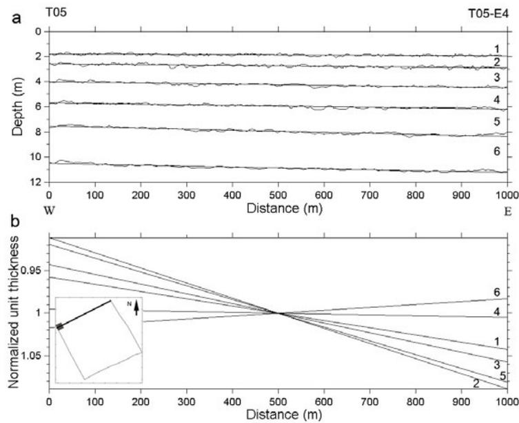
**Fig. 4.** (a) IRHs along the 1 km profile east of T05 (see inset in (b)). The positions of IRH centre lines and corresponding linear regression lines are plotted. (b) Normalized thickness for layers enclosed by adjacent horizons, with profile centres crossing the mean (normalized unit thickness  $\equiv 1$ ).
