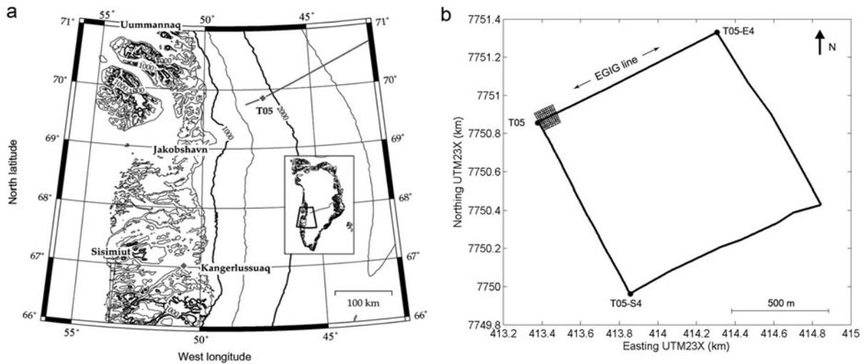
**Fig. 1.** (a) Map of the survey area around point T05 in the west-central region of the Greenland ice sheet. The line across the ice sheet indicates the position of the EGIG line. (b) Location of radar profiles near T05, forming a  $100\text{ m} \times 100\text{ m}$  grid with  $10\text{ m}$  spacing and a  $1\text{ km} \times 1\text{ km}$  square.
