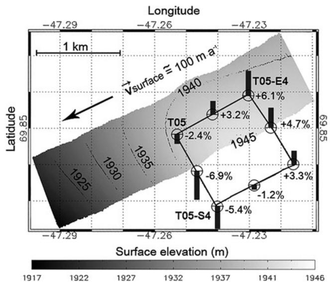
**Fig. 3.** Digital elevation model with 5 m contour lines, based on laser scanning during the ASIRAS campaign (Helm and others, 2007). Also shown is the location of the  $1\text{ km} \times 1\text{ km}$  square and the variation of cumulative mass above IRH-50 along its profiles. Bars visualize percentage deviations of inverse-distance weighted cumulative mass within a search radius of 100 m with respect to overall mean.
