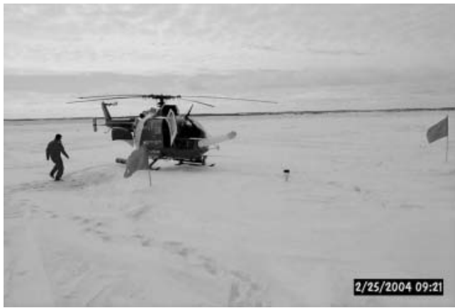
Fig. 2. Canadian Coast Guard helicopter on the Gulf of St Lawrence pack directly behind ice beacon 26 370. The EM/laser system can be seen fixed-mounted to the front of the helicopter.
