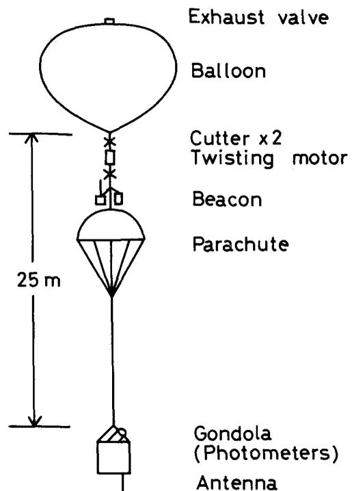
Figure 2. Construction of the Balloon.
