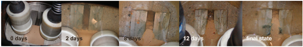
FIG. 4. The advance of bentonite into a fissure.
