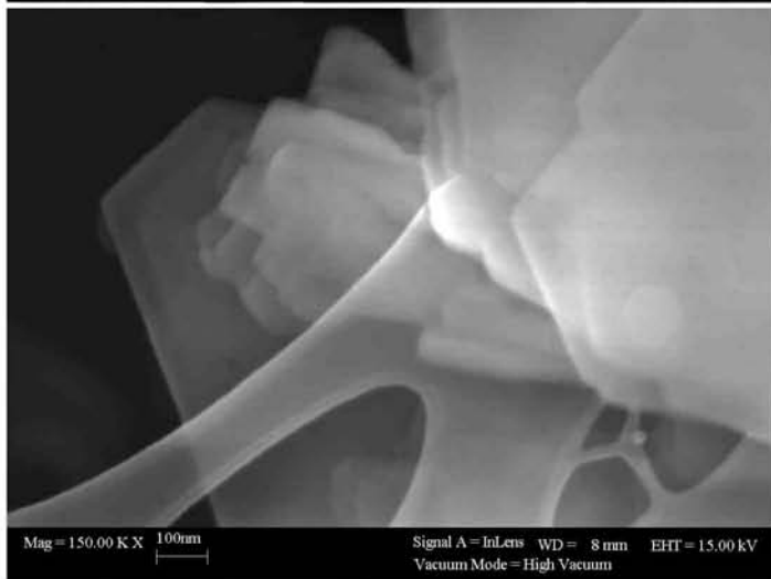
FIG. 1. (a-top) Low voltage SE image (0.3 kV) revealing (001) detailed surface features of kaolinite plates. (b) 15 kV voltage SE image showing 'transparent' kaolinite plates.
