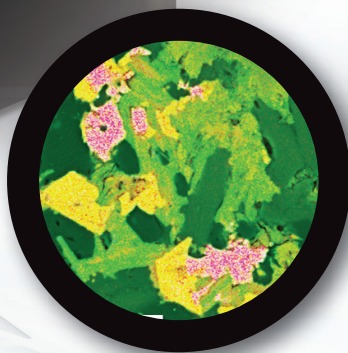
Geological thin section, elemental overlay 1 frame, 9.8 seconds
