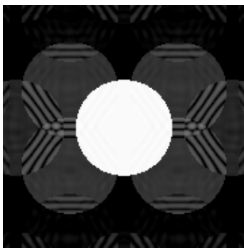
Fig.1. A simulated CBED pattern showing overlapping of the diffraction disks encoded the phase information.
