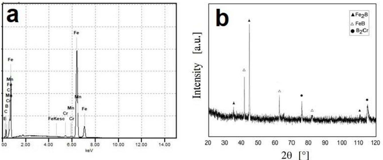
**Figure 2.** (a) Scanning EDS analysis for 9254 steel with DPB-9 and (b) XRD patterns obtained on 9254 steel exposed DPB-9.
