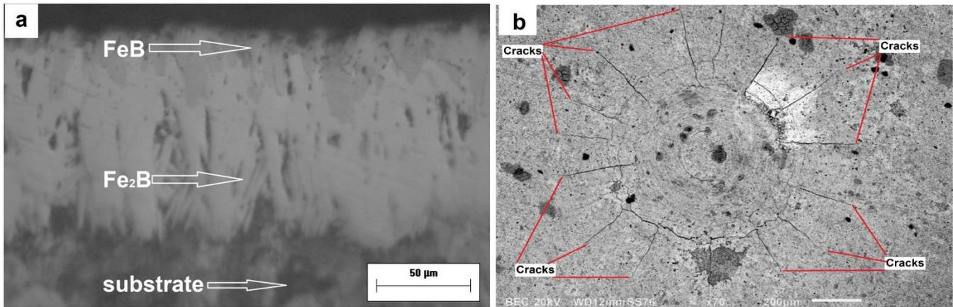
**Figure 1.** (a) Surface microstructure results on 9254 steel exposed to DPB-9 and (b) SEM images of the adhesion test for 9254 steel with DPB-9.
