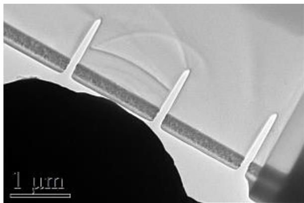
**Figure 1.** TEM image of the STM tip contacting the Ni/HfO<sub>2</sub>/Si ReRAM device
