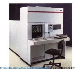
**RBS** can find it for you! **R**utherford **B**ackscattering **S**pectrometry– Quantitative atomic stoichiometry without standardization and nondestructive multi-layered depth profiling to 10,000Å.
