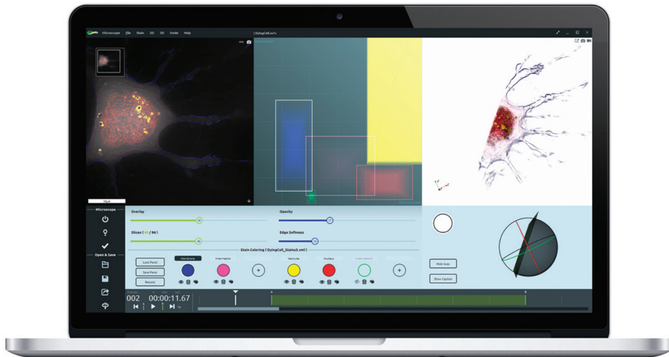
Figure 3: STEVE interface screenshot. The panel on the left offers a 2D viewer of the 96 z-stacks that compose the 3D image on the right. In the center, the Panel Viewer constitutes a fingerprint of the analyzed cell. In the x-axis refractive indexes are reported, while the y-axis shows the gradients. On the bottom (Control Field) the user can chose the color to apply to each cell part in order to produce the 3D reconstruction and modulate its transparency.
