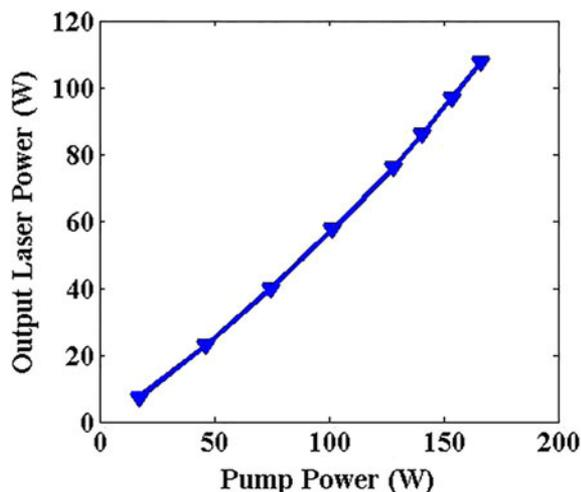
**Figure 2.** Laser output power versus pump power of the SFS-YDFL.
