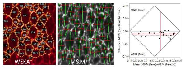
**Figure 2.** Matched pairs analysis of automatic cell size analysis with WEKA ("WEKA") and manual Measure and Mark method ("M&M") results.
