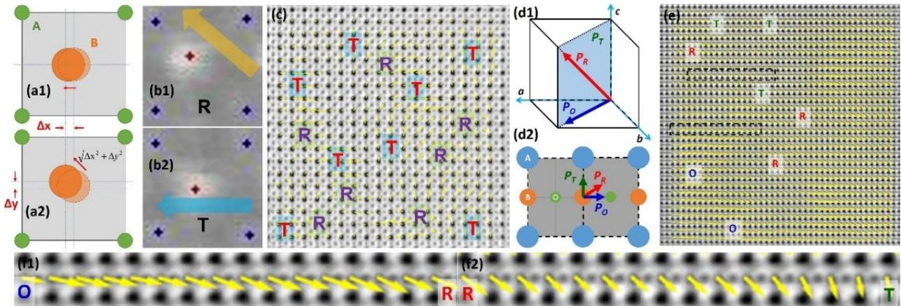
**Figure 1.** Structural models showing phase coexistence and gradual polarization rotation, (a1, a2) and (d1, d2); (b1,b2) STEM HAADF and (c) ABF images of KNN-based material with polarization map showing R+T phases; (e) ABF image of BT-based material with polarization map showing R+T+O; (f1,f2) Gradual polarization rotation between R, O, and T. Adapted from [2].
