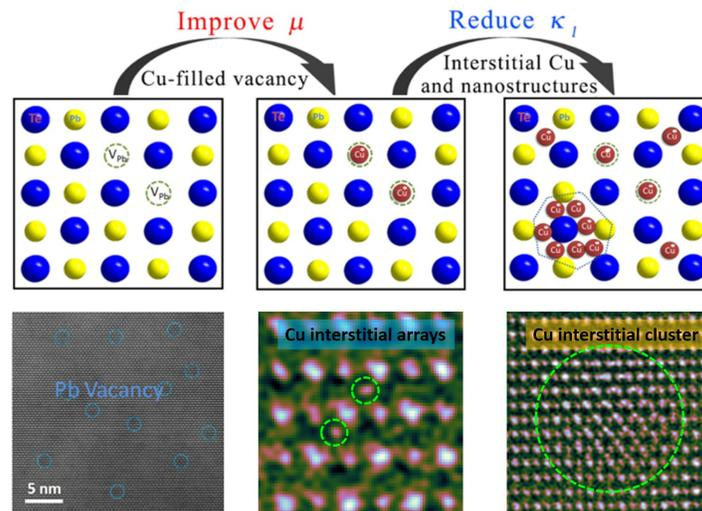
**Figure 2.** Schematic and structural evidence for the roles of Cu in PbTe: filling the intrinsic Pb vacancies to enhance carrier mobility and reducing the lattice thermal conductivity through scattering all-wavelength phonons via forming interstitials, clusters and precipitates. Reproduced from [4].
