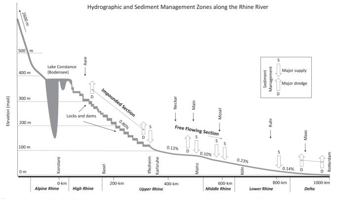
Figure 4.20. Longitudinal profile of the Rhine River, including geomorphic province, major tributaries, and sediment management operations. The stair-step pattern in the Upper and High Rhine is due to intensive impoundment. Gambsheim hydroelectric dam is located at 309-km, 25 km upstream of Iffezheim dam. (After Götz, 2008 and Frings et al., 2019.)
