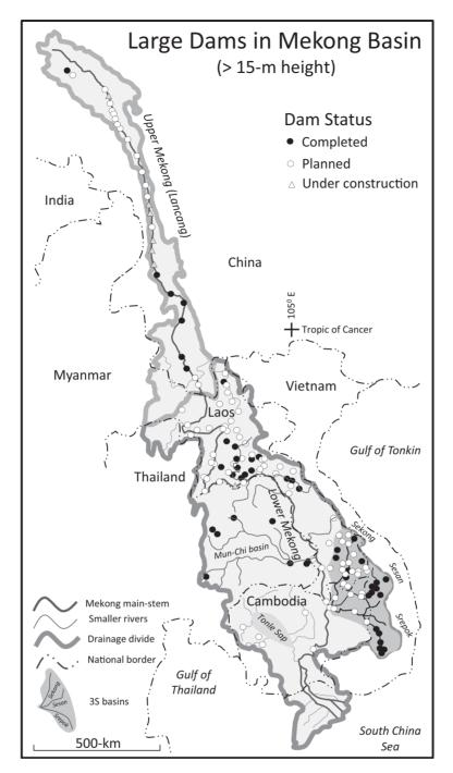
**Figure 4.19.** Location of large dams (> 15-m height) in the Mekong basin, including completed, under construction, and planned. The border between the Upper Mekong (Lancang) and Lower Mekong divide is indicated. The "3S" river basins refer to the Sekong, Sesan, and Srepok Rivers, which join to form the largest tributary in the lower Mekong. (Author figure. Data sources include Mekong River Commission and Räsänen et al., 2017 (for large dams).)
