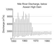
**Figure 4.15.** Streamflow variability of Nile River below Aswan Dam between 1950 and 1985, revealing impacts to annual flood pulse (higher low flows, much lower peak flows) after dam closure over 1965–1967. (Figure Source: Vörösmarty and Sahagian, 2000).
