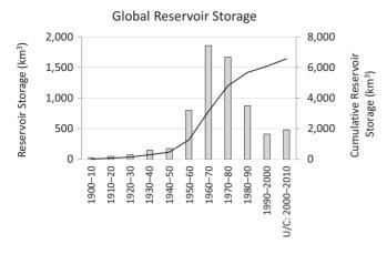
**Figure 4.4.** Global growth of reservoir storage capacity between 1900 and about 2010, including dams under construction and planned (U/C) between 2000 and 2010. (Source: Walling, 2006.)
