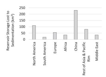
**Figure 4.45.** The global distribution of reservoir storage lost to sedimentation. (Figure source: Walling, 2006.)
