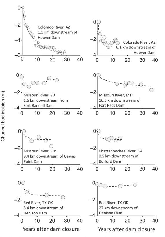
Figure 4.25. Channel bed adjustment for several US rivers, with river and station names relative to distance downstream of dams (on figure). (Data: Williams and Wolman, 1984.)
