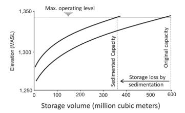
**Figure 4.46.** Reservoir elevation-storage: Comparison of original relationship and curve shift and storage volume lost due to reservoir sedimentation. (Source: Annandale et al., 2016.)
