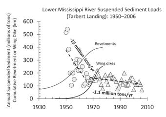
**Figure 4.24.** Historic change to suspended sediment loads for the lower Mississippi River at Tarbert Landing, Louisiana. Trend lines coincide with years 1950–1967 (-15 million tons/yr) and 1968–2006 (-1.1 million tons/yr). Cumulative distance (km) for revetment and wing dike (groyne) construction included for USACE Memphis and Vicksburg Districts. (Source: Meade and Moody, 2010.)
