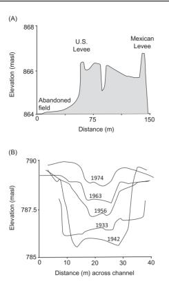
**Figure 4.27.** Changes to Rio Grande/Bravo at Presidio, Texas/Ojinaga, Chihuahua. (A) Deposition between the levees (dikes) resulting in embanked floodplain aggradation. (B) +3 m of channel bed aggradation and narrowing due to reduced flow conveyance caused by upstream impoundment and water withdrawal. (Source: Collier et al., 1996, data from Everitt, 1993.)
