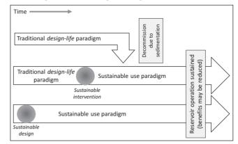
**Figure 4.53.** Models of dam and reservoir design related to sediment management. Conventional "design-life" paradigm for dams and reservoirs can be modified toward a sustainable use paradigm. New dam construction should include features adaptable to changing sediment management strategies. (Source: Annandale et al., 2016.)
