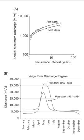
**Figure 4.12.** Changes to flow regime for two large European rivers, before and after impoundment. (A) Reduction in annual maximum floods, lower Ebro River (at Tortosa) downstream of the Mequinenza and Ribarroja reservoirs. (B) Changes to lower Volga River discharge regime after dam closure over 1959–1960. (Sources: Ebro River, Batalla, 2003; Volga River, Schmutz and Moog, 2018 with data from Górski et al., 2012.)
