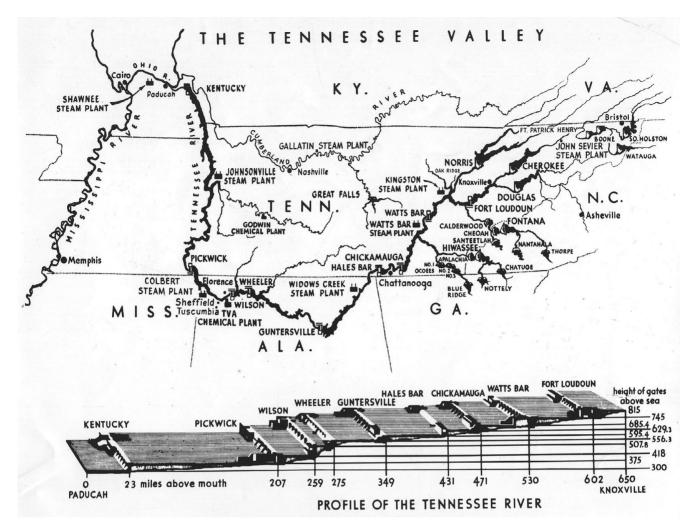
Figure 4.35. Map of the profile of the Tennessee River, showing locations of TVA dams and drainage network of the Tennessee River basin. Unit conversion: 1 mile = 1.6094 km, 1 ft = 0.3048 m. (Source: Tennessee State Library and Archives.)
