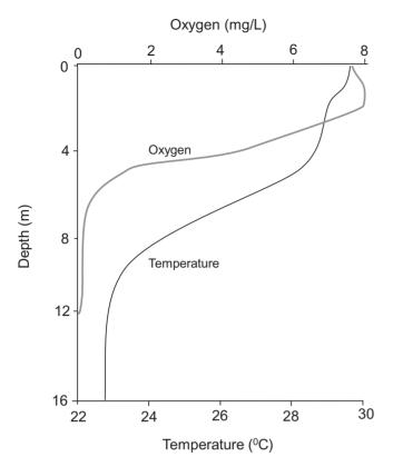
**Figure 4.33.** Reservoir depth (m) profile for water temperature (C) and dissolved oxygen (mg/L) in 2004 for stratified Nam Leuk Reservoir, Laos, Mekong basin. (Source: Hortle and Nam, 2017.)
