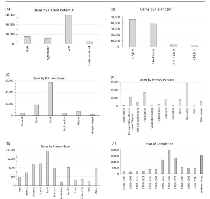
**Figure 4.8.** The United States has 91,457 dams (A) decade of completion, (B) height, (C) primary purpose, (D) primary owner, (E) primary type, and (F) hazard potential. Note: y-axis for dam type (E) is logarithmic. (Author figure. Data source: U.S. Army Corps of Engineers National Inventory of Dams.)
