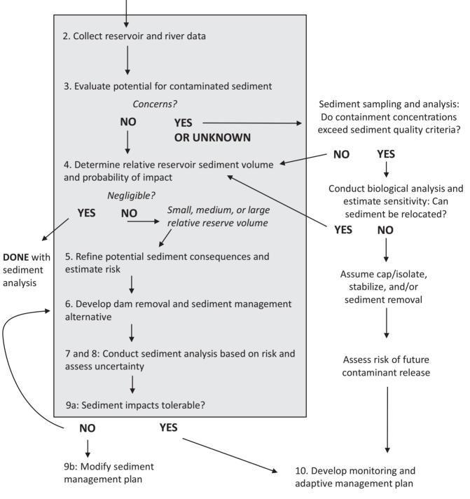
Figure 4.38. Steps for removal of reservoir sedimentary deposits. Sequence largely depends upon environmental concerns related to reservoir deposits. (Source: Randle et al., 2019.)
