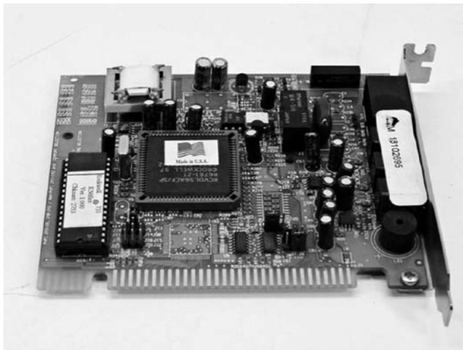
FIGURE 5.4 A Rockwell 33.6 K analog modem, c.1990s.
