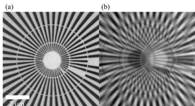
**Figure 1.** Observed image of a resolution test chart with the innermost line width of 50 nm. (a) Absorption image and (b) twin phase image. The gray scales of the image correspond to  $-1.2 - 1.2$  in phase shift (radian).
