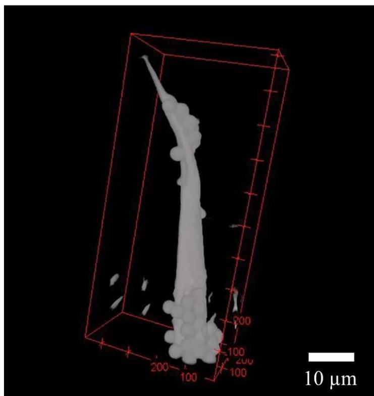
**Figure 3.** X-ray phase-CT image (volume rendering) of polystyrene spheres (diameter: 3  $\mu\text{m}$ ) on a plastic fiber obtained by 360 CT projections. Single projection image was obtained by phase stepping measurement of 6 step with each exposure time of 20s.
