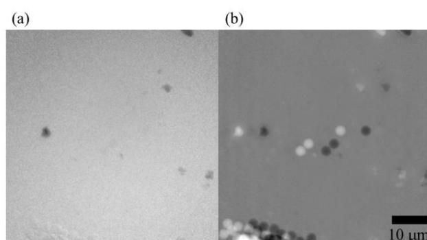
**Figure 2.** Comparison of observed image of polystyrene spheres (diameter: 3  $\mu\text{m}$ ). (a) Absorption image and (b) twin phase image. The gray scales of the images correspond to (a)  $0.95 - 1.01$  in transmittance and (b)  $-1 - 1$  in
