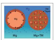
Particles of pure magnesium (left) can only collect a limited amount of hydrogen on their outer surfaces. and the process is slow. But when the magnesium is doped with iron (right), far more hydrogen is delivered through the iron layers, which also results in much faster charging. *Credit:* NIST
