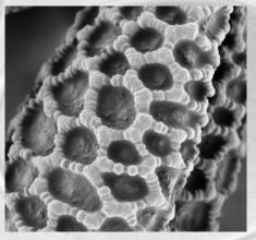
Surface of uncoated pollen, imaged using SEM at very low kV (50 V).
