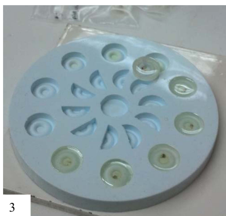
Figure 3. Samples less 3mm were embedded in epoxy resin which were polished for optical and SEM-EDS analysis in cross-section. Figure 4. Cross-section of a painted earthen plaster shows three layers of paint as well plaster substrate (FSC-A-11)
