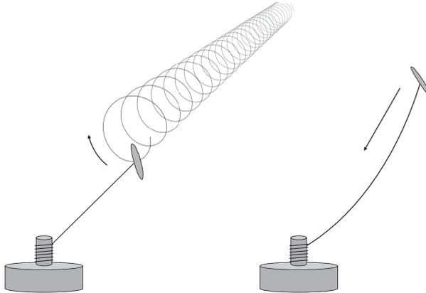
Figure 1.3 Simplistic view of a kite connected to a drum, with an indication of the flying pattern when power is produced (left) and when flying back (right).
