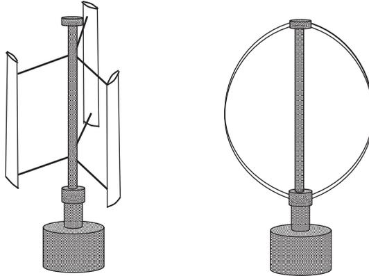
Figure 1.2 Vertical-axis wind turbines. “H-shaped” type (left) and Darrieus (“eggbeater”) type (right).
