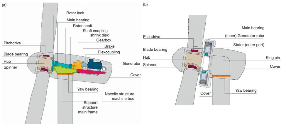
Figure 1.1 Illustration of the main components in a geared wind turbine (left) and a direct-drive turbine (right). Reproduced with permission of Fraunhofer IWES. Source: Wenske (2022).
